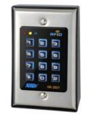
The DK-2821 is a self-contained single relay output keypad. It combines the functions of digital keypad and proximity EM card reader in one unit. The buttons of the keypad are epoxy coated silicone rubber that is prepared for high traffic access control applications.
