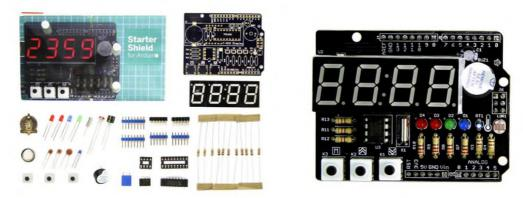
Starter Shield is a perfect start for beginners of Arduino world. You can learn and practice basic soldering tricks and programming principles when tinkering with this kit. Electronic could be fun even if you have bare technical knowledge cause we get your back by preparing a detailed soldering guide and a fully supported library of programming examples from easy to difficult. Hope you have fun and gain some knowledge with this kit!
